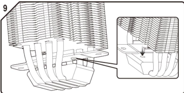
Cross the crossbar through above the Heat-sink base, and aim the raise points of crossbar to holes of Heat-sink base.
