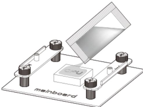
Please clean the surface of CPU before applying the thermal grease, then apply thermal grease evenly on CPU.
