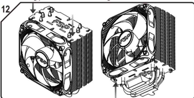
Insert anti-vibration rubbers into Heat-sink(insert through from top of fins) Then, insert anti-vibration rubbers into Heat-sink (insert through bottom of fins)
