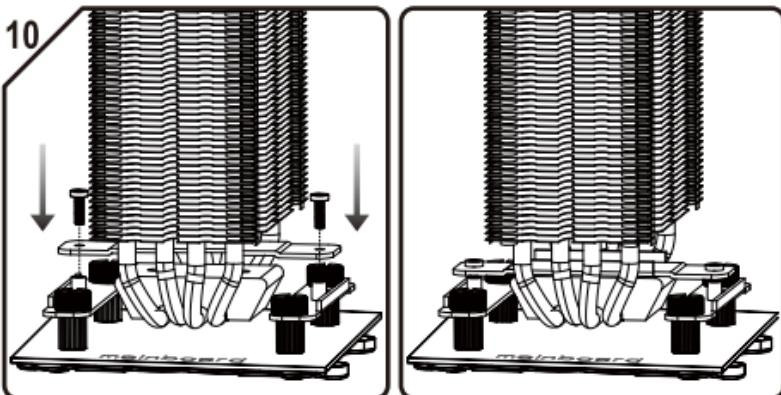
Aim the holes of crossbar to the pillar holes of mounting-clip, then use screw driver and M3 screw to fasten cross bar and mounting-clips.
