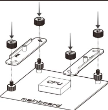
Aim the holes of Intel mounting-clip to the LGA 2011 screws, and slip over the clips to the screw. Then fasten the metal nuts onto LGA 2011 screws.
