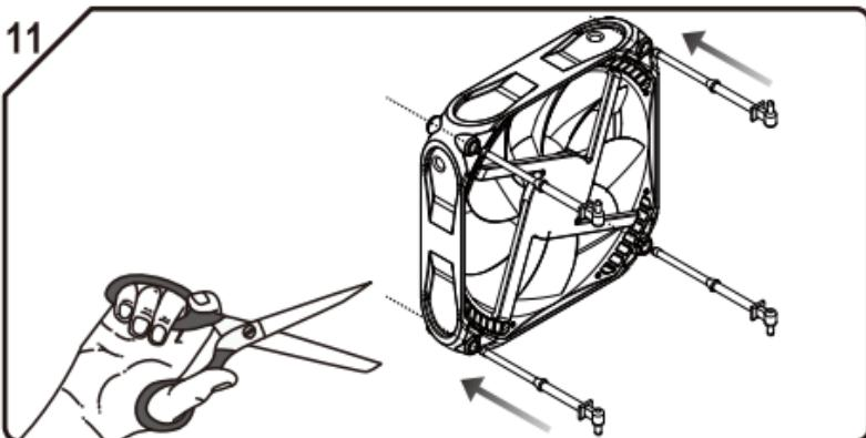
Securely fix the anti-vibration rubbers onto the fan. (2 sets of rubbers, 8 pieces in total, are included. Handle of rubber to direction under.) To keep the fan clean and tidy, you can cut off the outstanding part of rubbers after fixing them onto the fan.
